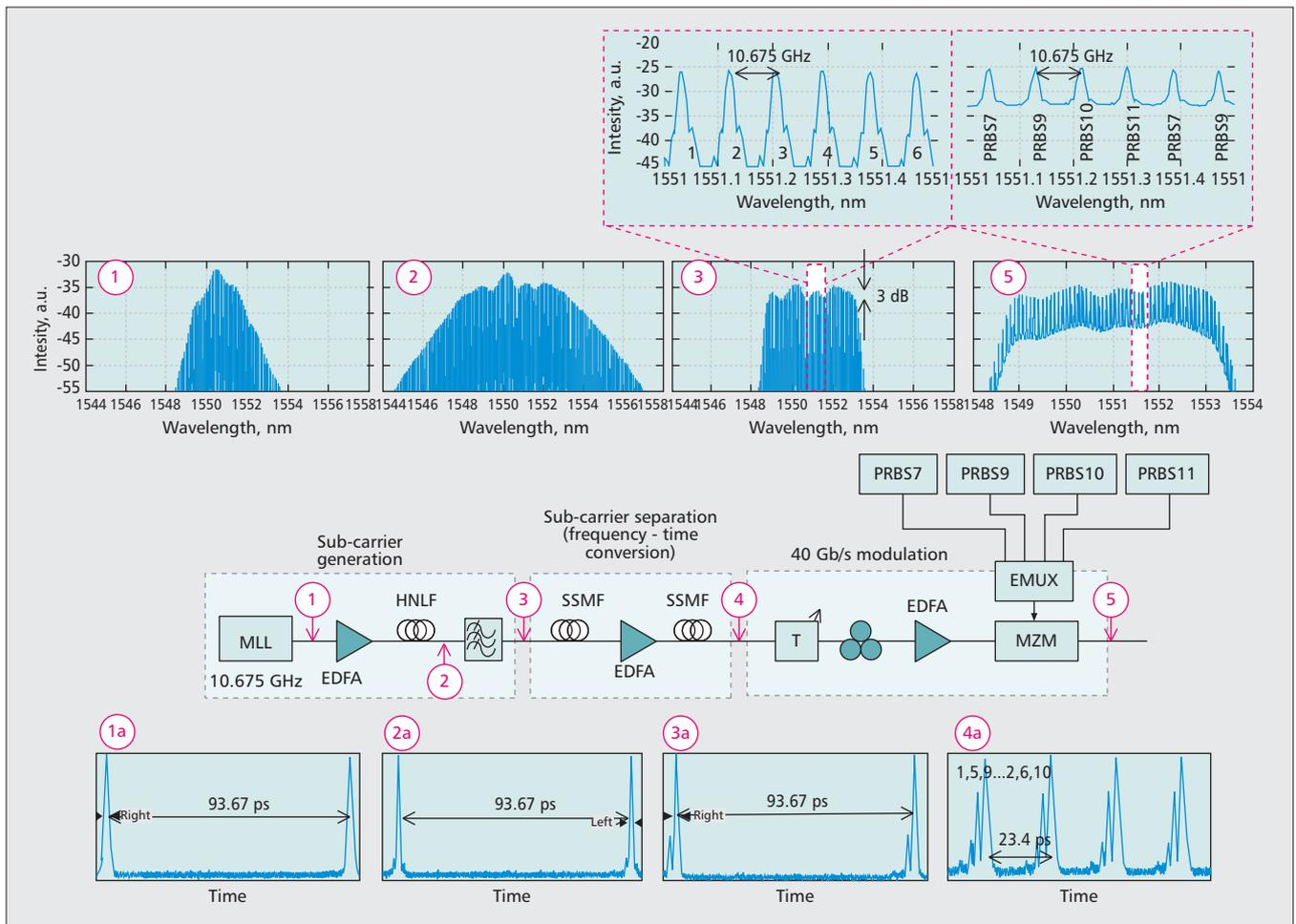
**Figure 2.** Experimental setup of a 555 Gb/s optical comb generator. PRBS: pseudo-random binary sequence; EDFA: Erbium-doped fiber amplifier; EMUX: electrical multiplexing; MZM: Mach-Zehnder modulator.
