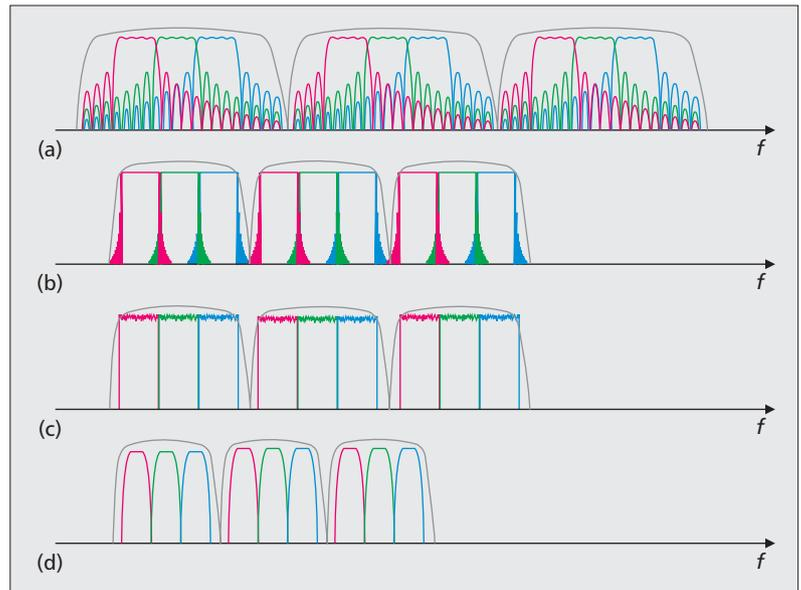
**Figure 4.** Illustrative examples of spectrum for OFDM with a) 4 subcarriers and b) 256 subcarriers; c) NWDM; d) TFP.
