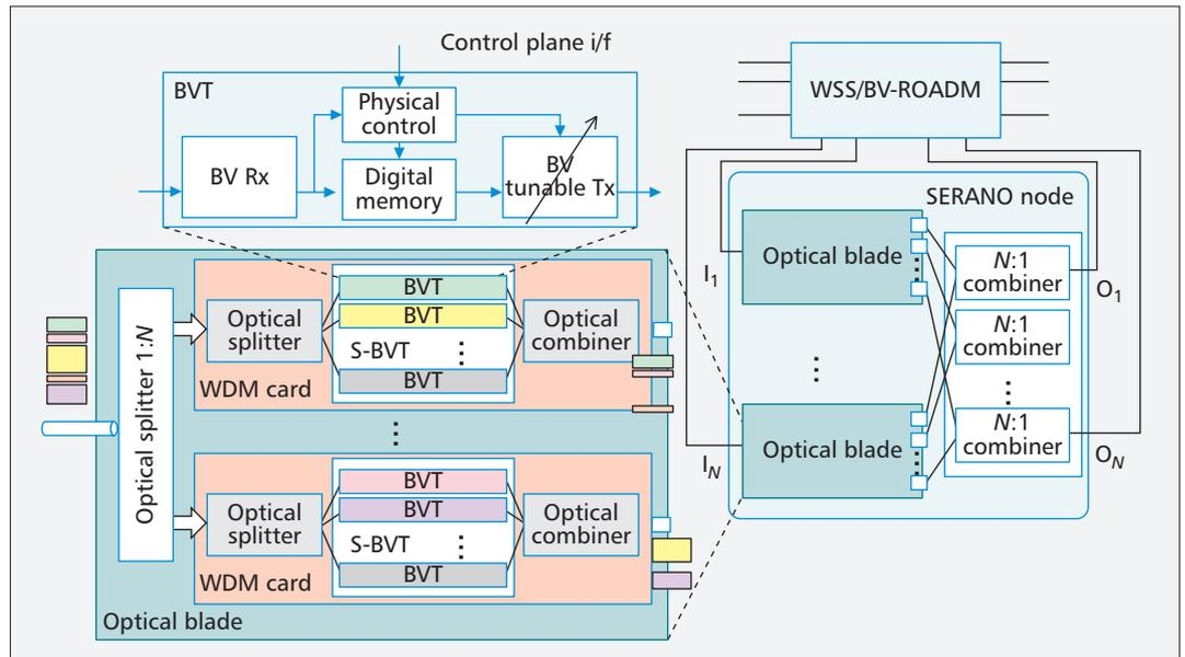
Figure 3. Overview of the SERANO architecture with simplified S-BVT modules embedded.
