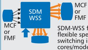
MCF or FMF<br>SDM-WSS for joint flexible spectral channel switching in multiple cores/modes (see [6])                                                                                           |
