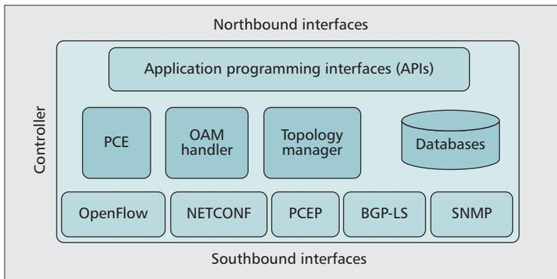
**Figure 6.** Converged ABNO and SDN controller architecture including the most relevant modules and interfaces.
