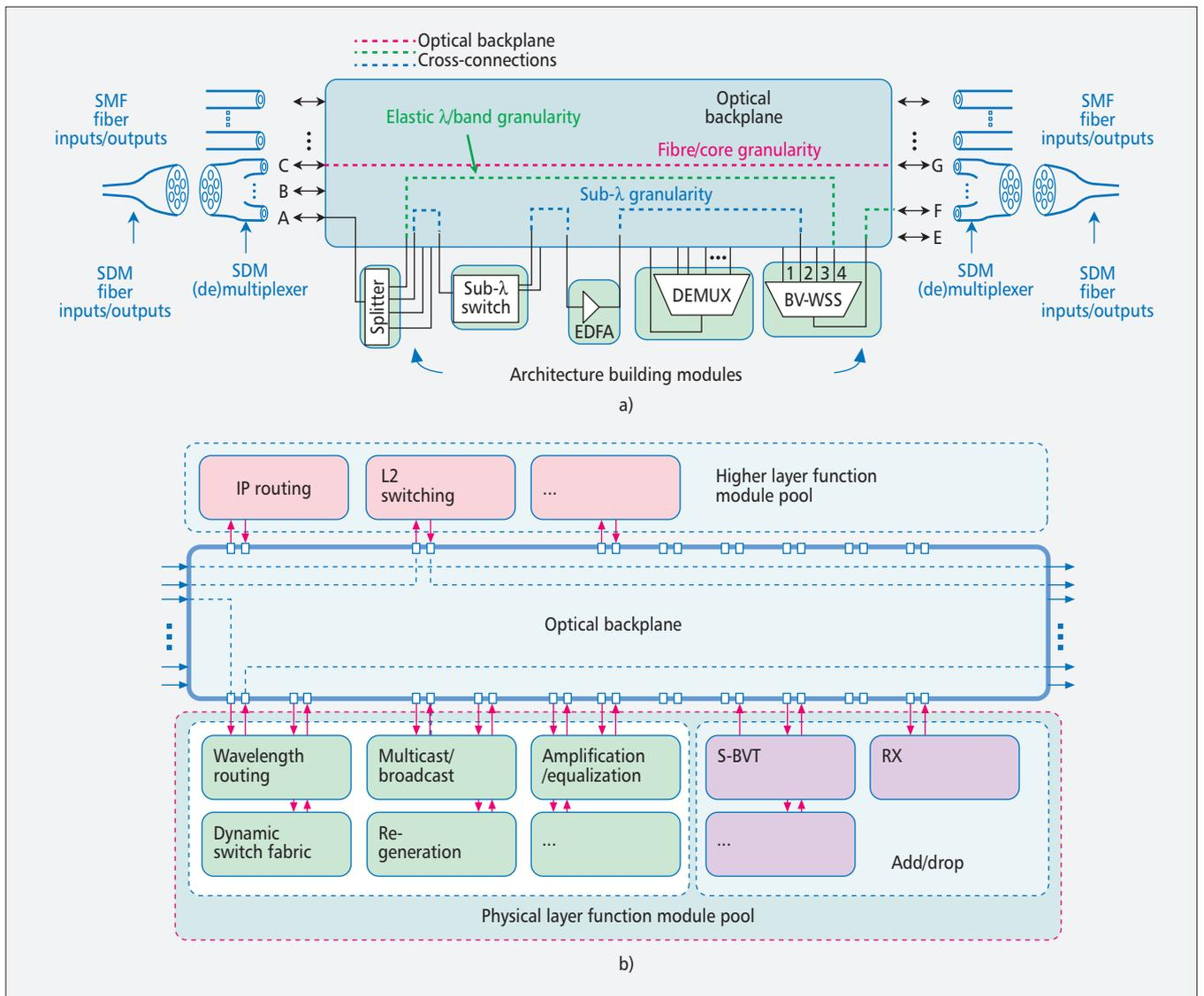
Figure 2. a) AoD-based Flex-OXC node; b) Flex-OXC node supported by NFP.
