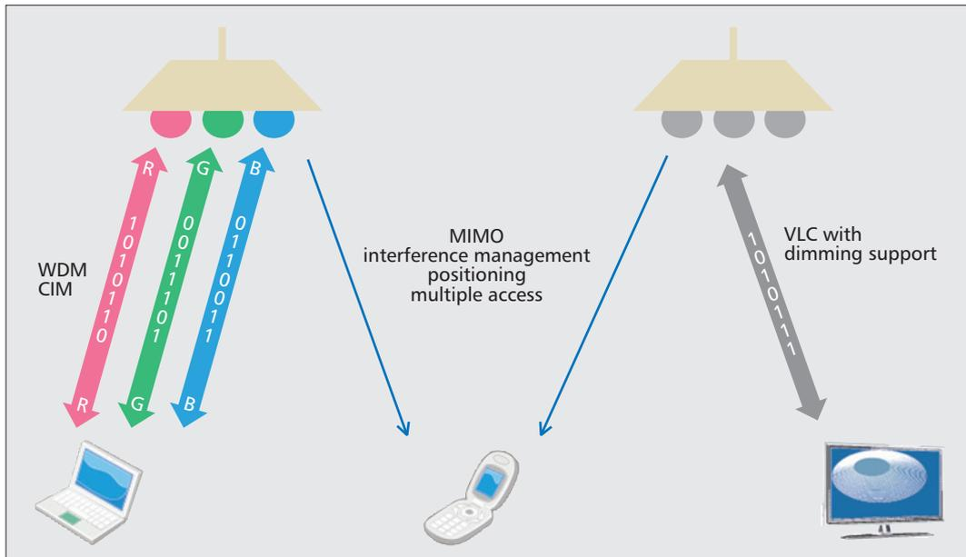
**Figure 1.** Configurations of VLC. VLC can be configured in various ways according to the configuration of the LED lamps: a single data stream transmission via a single PC LED, multiple data stream transmission via an array of RGB LEDs, and so on.
