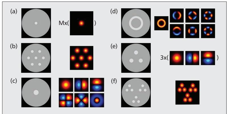
**Figure 1.** Different types of fibers in support of SDM, showing their geometrical form and propagating spatial mode distributions: a) single-mode fiber array; b) multi-core fiber; c) few-mode fiber; d) annular-core fiber; e) multi-core supporting few modes; f) multi-core arranged in coupled subgroups.
