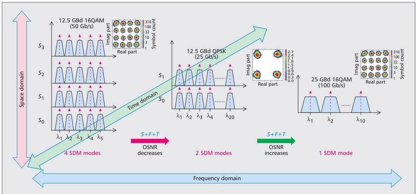
**Figure 2.** Three different possibilities to provision a 1 Tb/s connection exploiting flexibility in space, frequency, and time (S+F+T).
