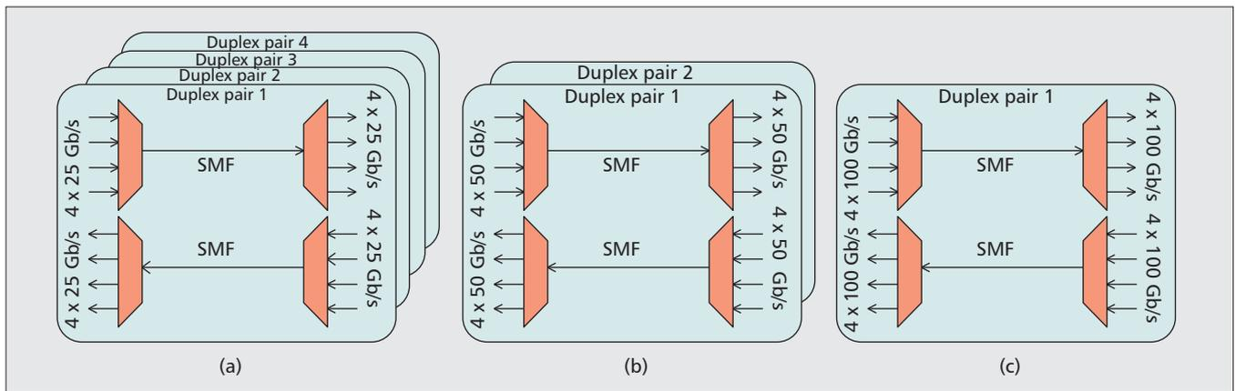
**Figure 2.** 400 GbE solutions with different numbers of lanes with different bit rates per lane.
