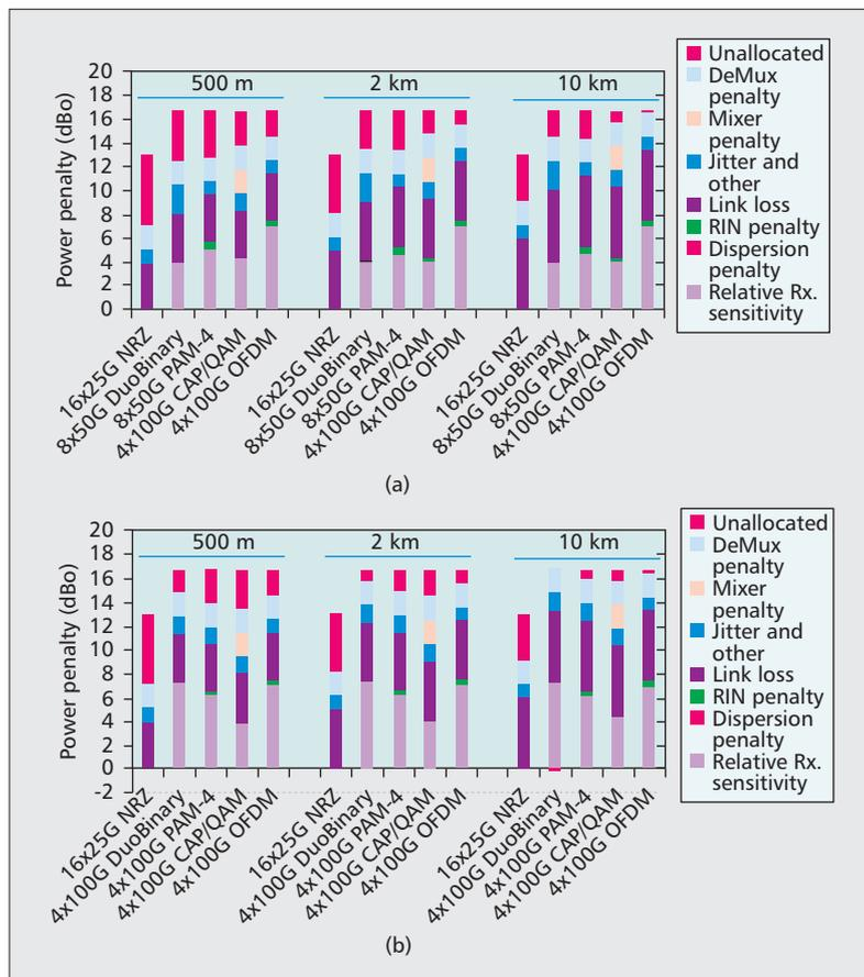
**Figure 5.** Link optical power penalties for various 400 GbE links using different modulation formats under: a) DML case; b) EML case.
