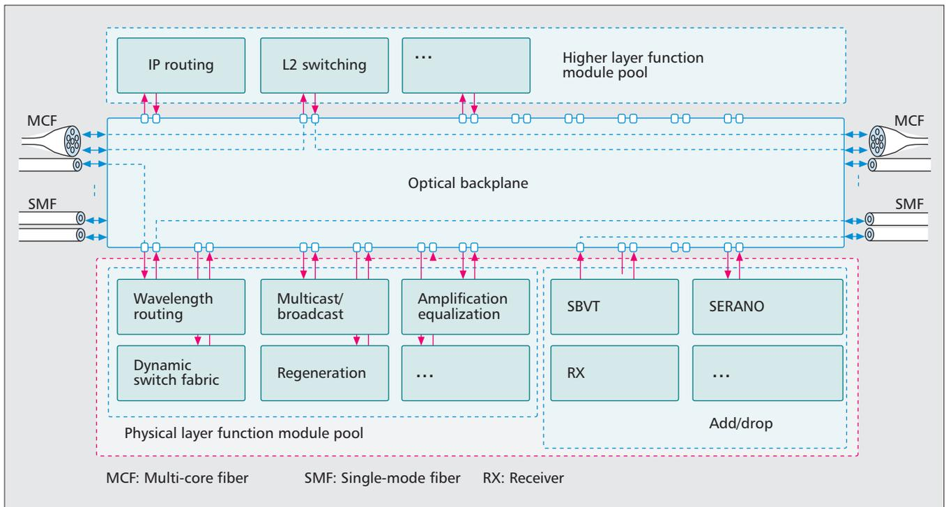
Figure 3. AoD-based NFP node.
