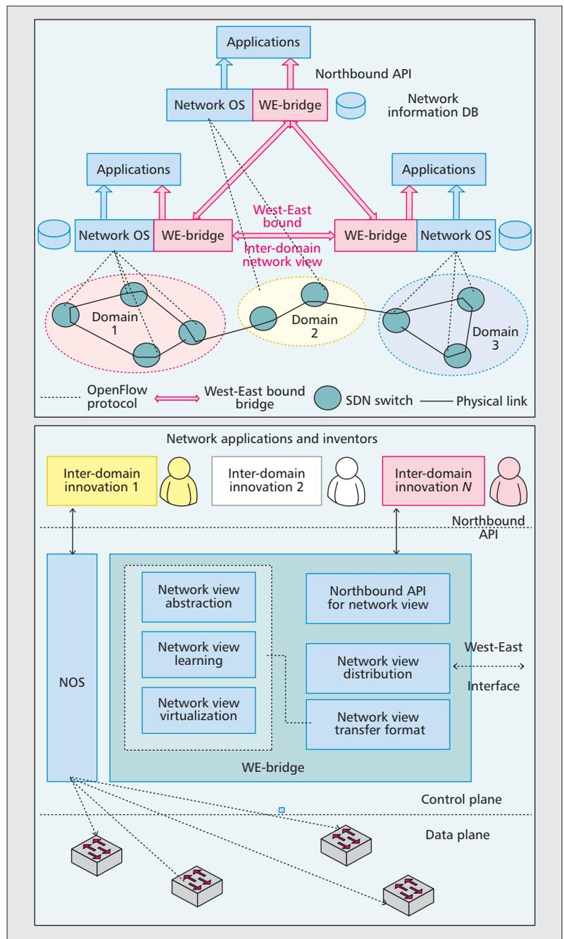
Figure 1. West-East Bridge for SDN inter-domain communication (top); overview of WE-Bridge (bottom).
