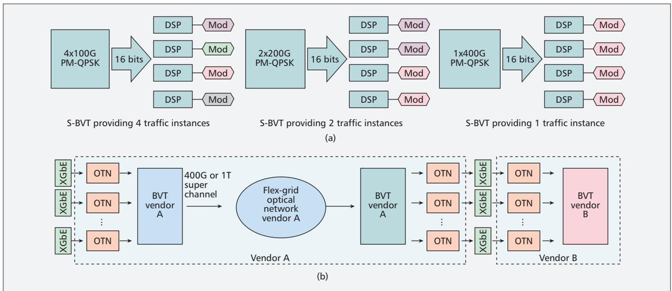
**Figure 4.** a) Example of S-BVT adaptation in regard to a variable number/size of traffic instances; b) multivendor interoperability using standardized interfaces.
