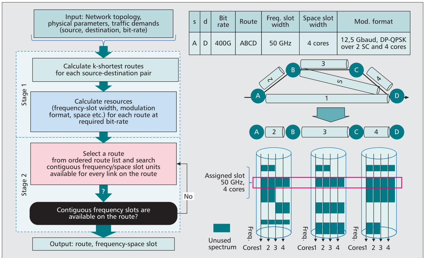
**Figure 3.** An example of the process and the main calculation steps for identifying and assigning a capacity demand in a flexible network.
