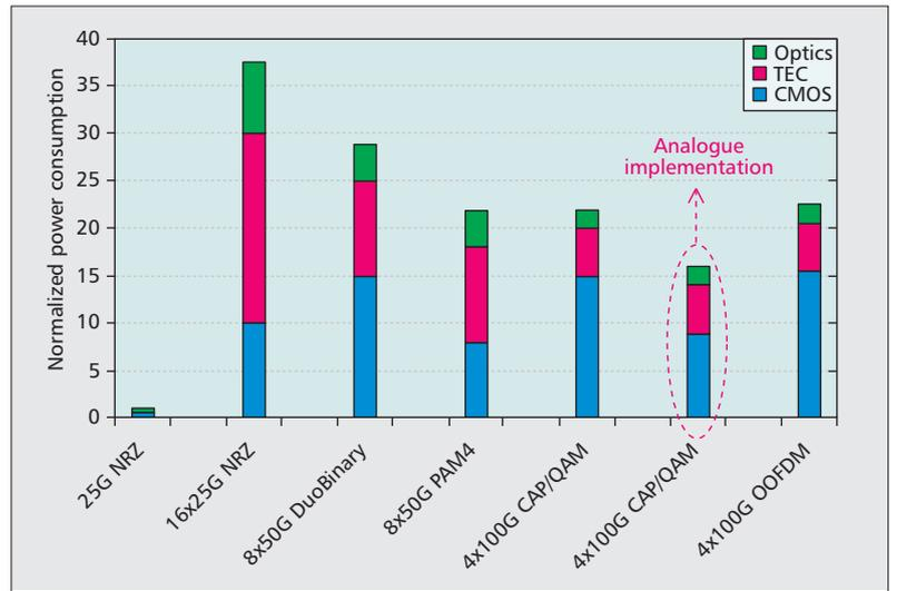
Figure 6. Estimated power dissipation of various SMF transceivers to support 400 Gb/s bit rate.
