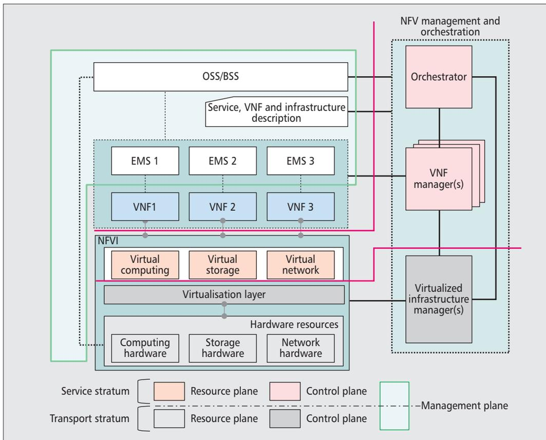
**Figure 5.** Layered approach to NFV control.
