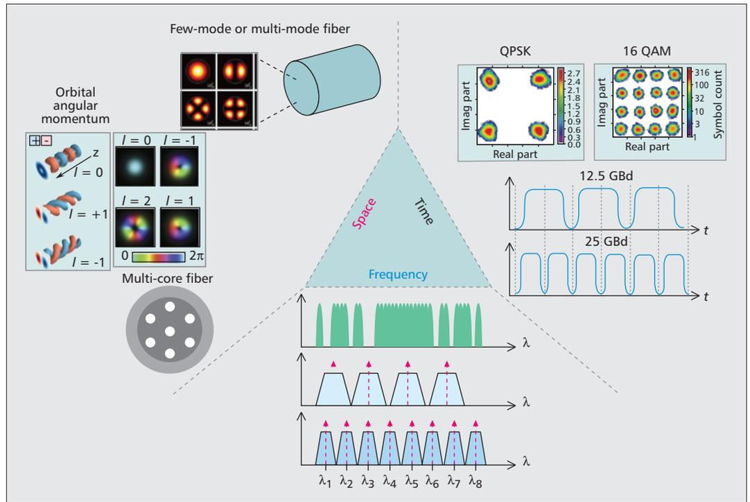
**Figure 1.** Three physical domains (frequency, time-modulation format, and space) to support elastic optical networking in the spectral, temporal, and spatial domains (3D-EON).
