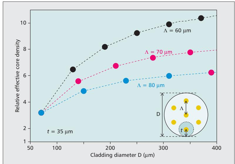
**Figure 1.** Geometrical relationship between relative effective core density and cladding diameter when  $t = 35 \mu\text{m}$ . Black, red, and blue plots show the results when  $\Lambda$  was assumed to be 60, 70, and 80  $\mu\text{m}$ , respectively.
