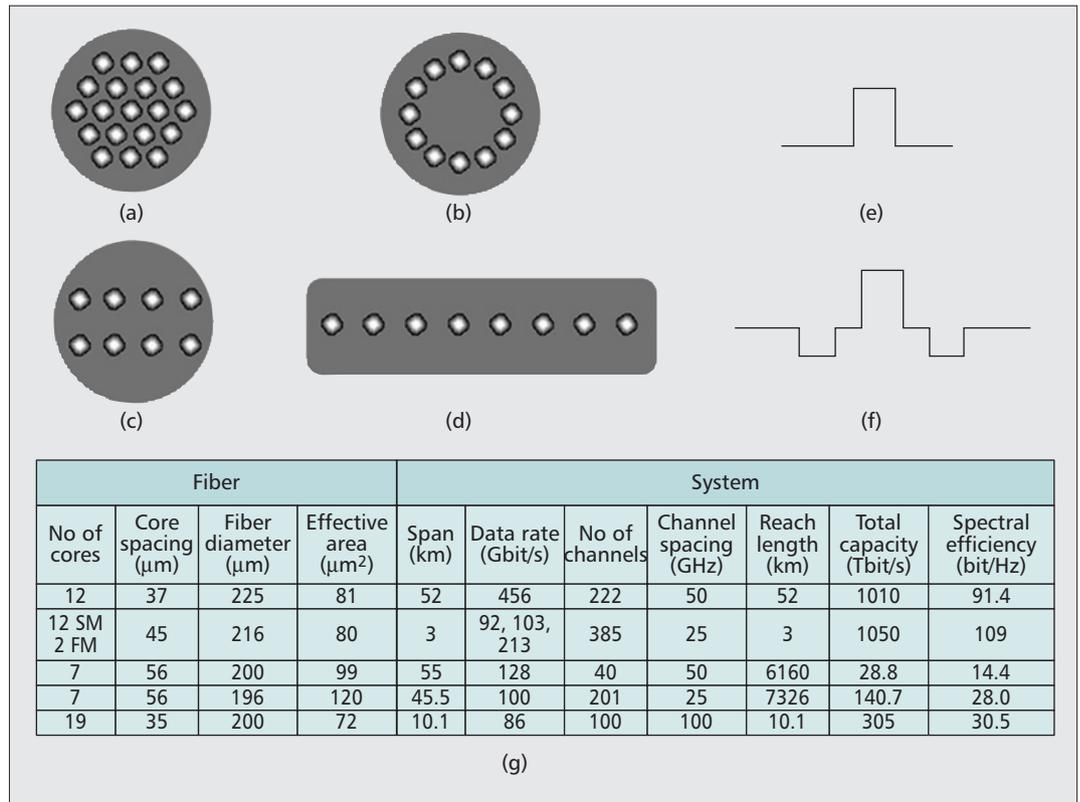
**Figure 4.** Multi-core fiber designs (a–d), refractive index profiles (e–f), and the most recent SDM transmission experiments using MCF (g).
