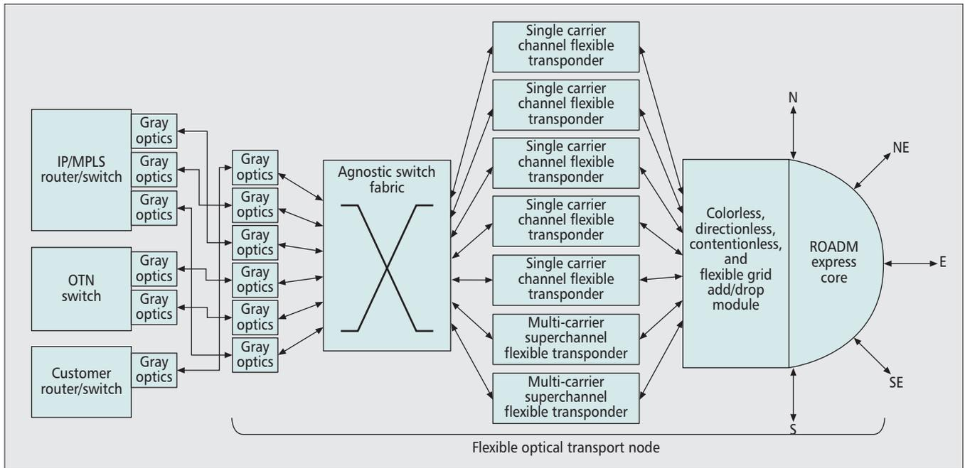
**Figure 3.** An example of a flexible optical transport node with agnostic switch fabrics, coherent channels, and CDC-F ROADM.
