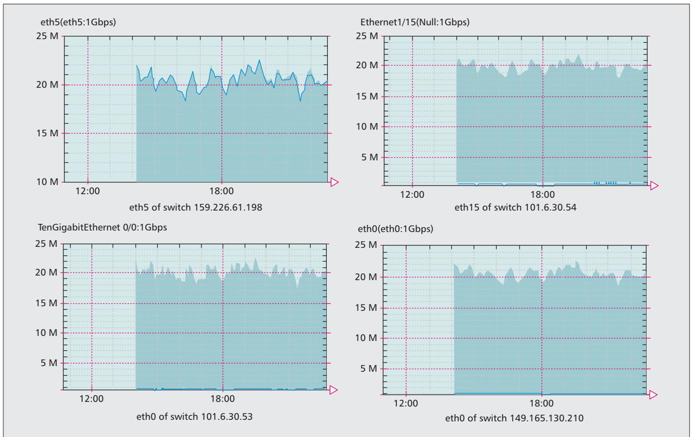
Figure 5. Traffic at interfaces of OpenFlow switches along the routing path.
