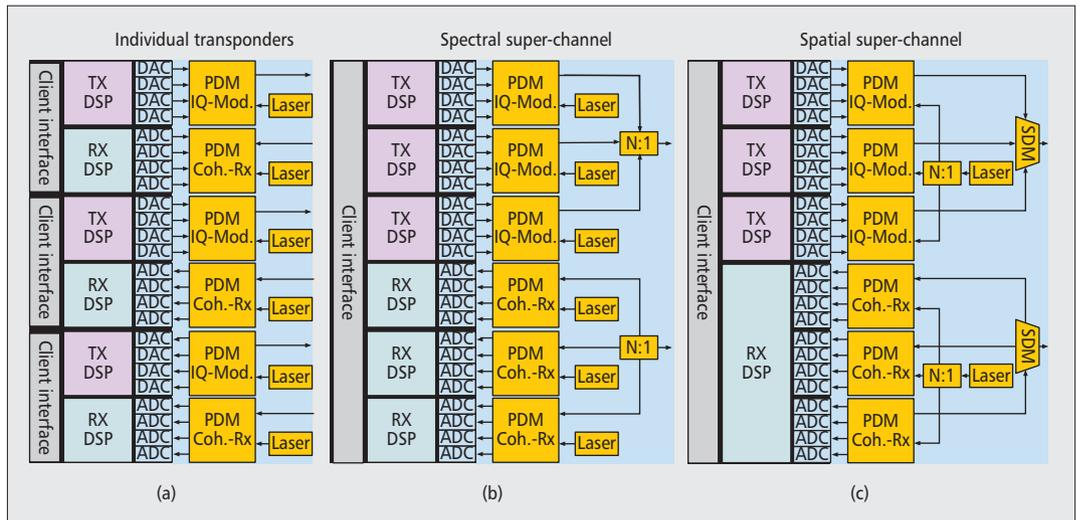
**Figure 1.** Examples of super-channel architectures with three subchannels: a) individual transponders; b) spectral super-channel transponder; c) spatial super-channel transponder.
