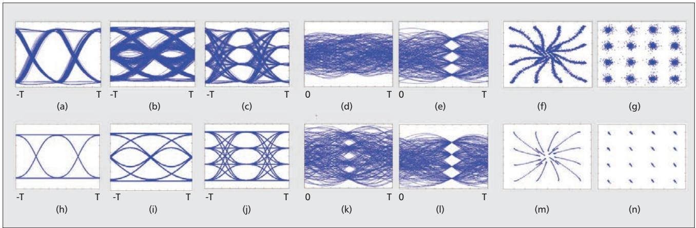
**Figure 4.** 4 Representative eye diagrams and constellation diagrams for 25 Gb/s NRZ, 50 Gb/s duobinary and PAM-4, and 100 Gb/s hybrid CAP-16/QAM-16 and QAM-16-OFDM. (a–g) are for the DML case; (h–n) are for the EML case.
