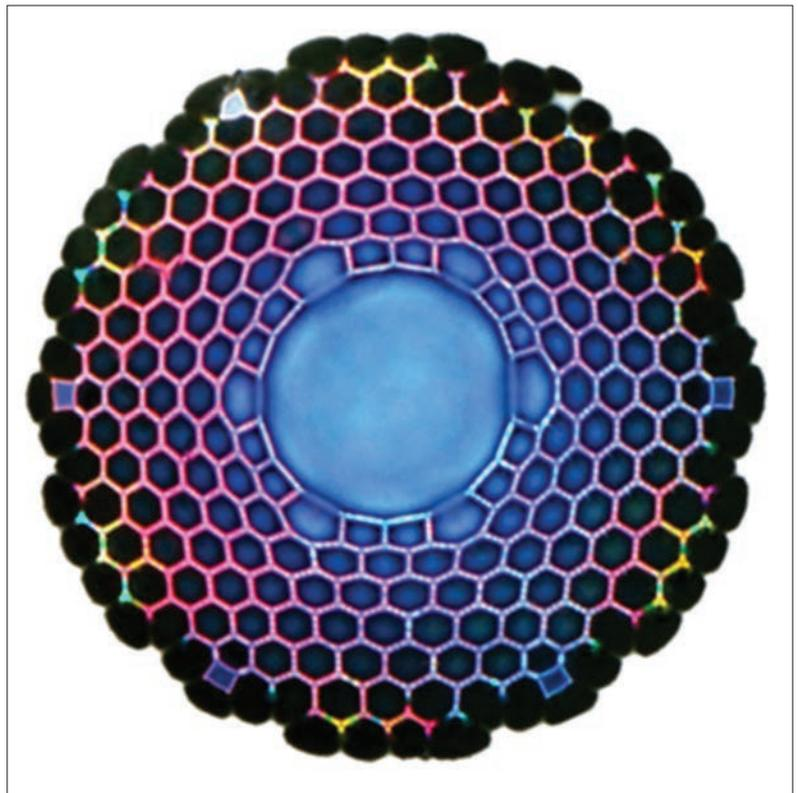
**Figure 3.** Microscope image of a typical large core HC-PBGF under white light illumination conditions. (Figure courtesy of S.R. Sandoghchi, Optoelectronics Research Centre, University of Southampton.)
