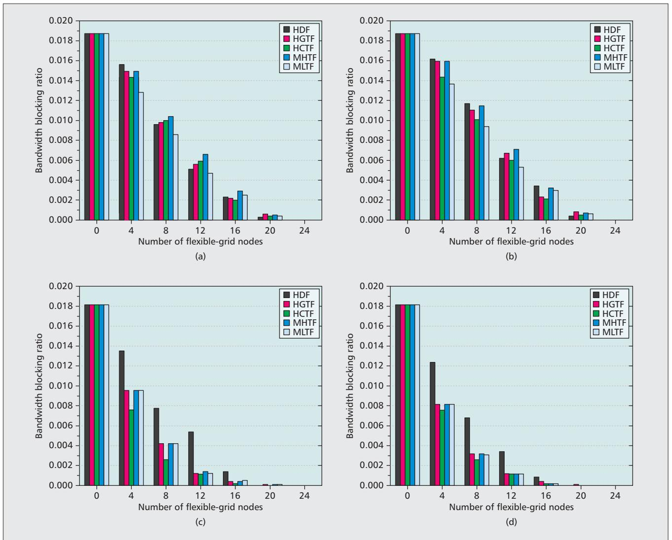
**Figure 3.** Bandwidth blocking ratio for traffic profile 1: a) forming one island under uniform traffic; b) forming two islands under uniform traffic; c) forming one island under non-uniform traffic; d) forming two islands under non-uniform traffic.
