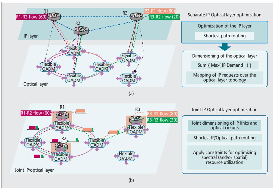
**Figure 5.** Multi-layer network planning approaches: a) the current approach, which treats IP and optical layers separately, providing optimized IP flow routing and then mapping of requests over optical layer topology; b) the joint IP-optical layer optimization approach, in which IP routing and optical resources are jointly considered and optimized for each demand.
