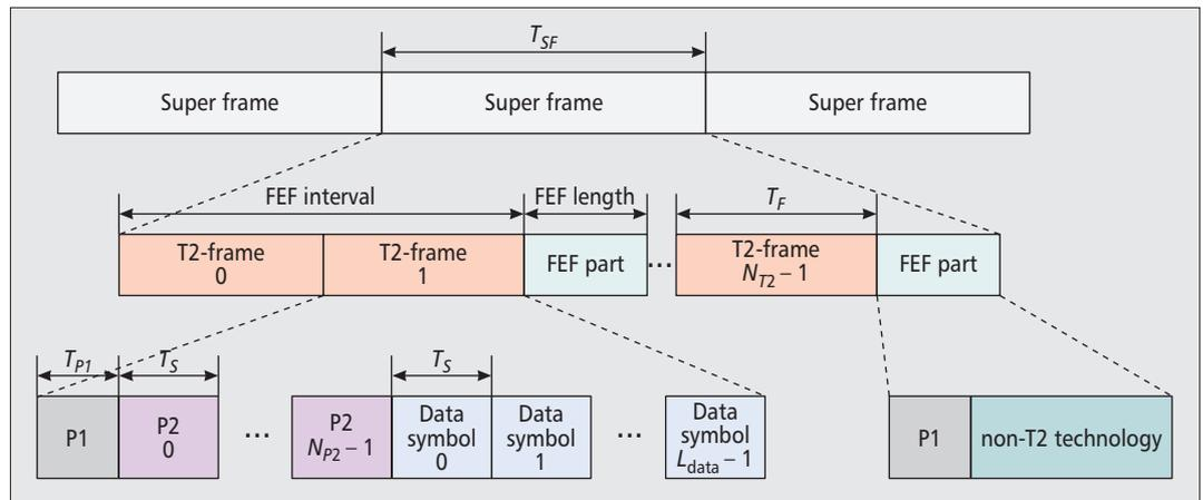
Figure 3. The DVB-T2 frame structure, showing the division into super-frames, T2-frames and FEF.
