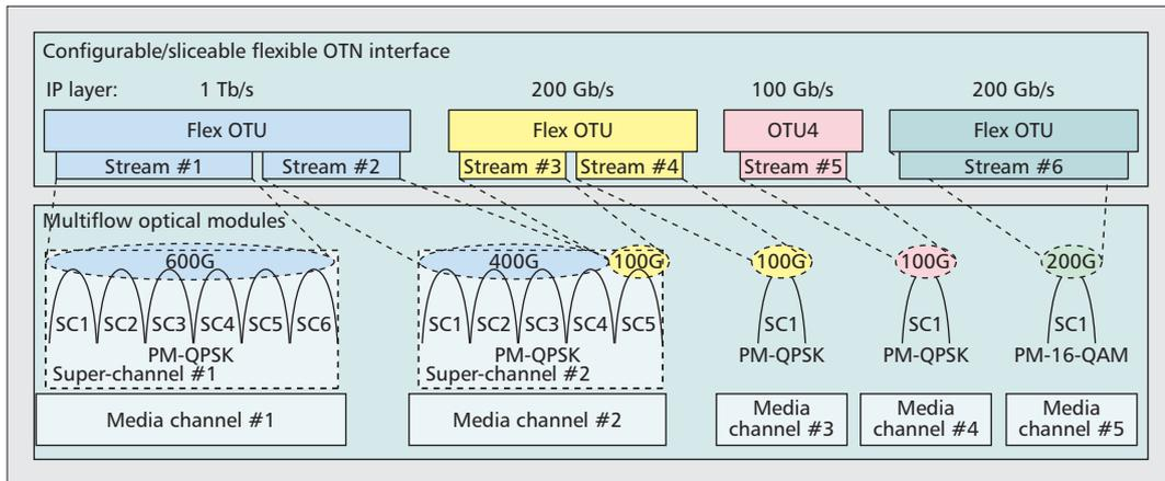
**Figure 2.** OTN frames and flexible association with media channels.
