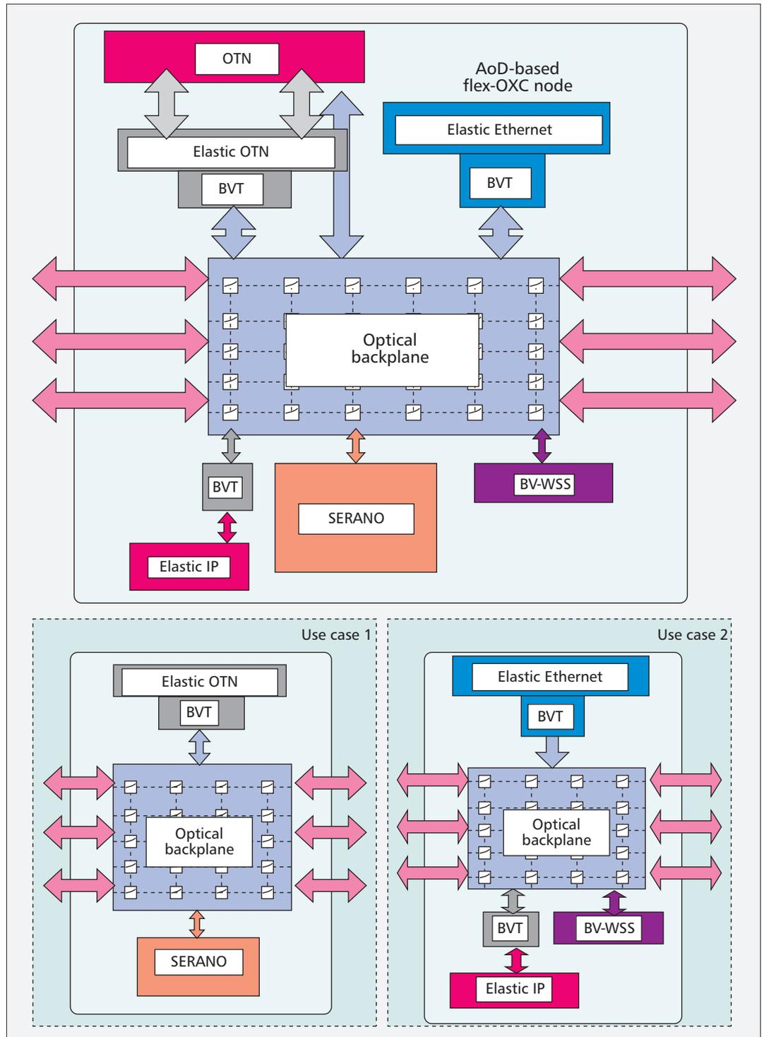
Figure 1. Flex-OXC node adaptability to different use cases.
