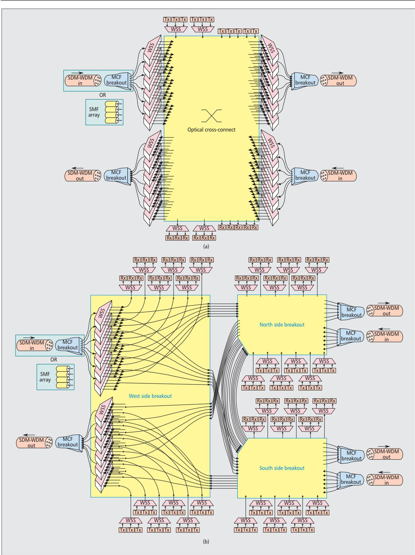
**Figure 3.** Implementations for independent spatial mode/wavelength channel switching: a) optical cross-connect for full connectivity (only two fiber links shown); b) route-and-select per each spatial mode. North and south side breakouts are identical to the west side breakout.
