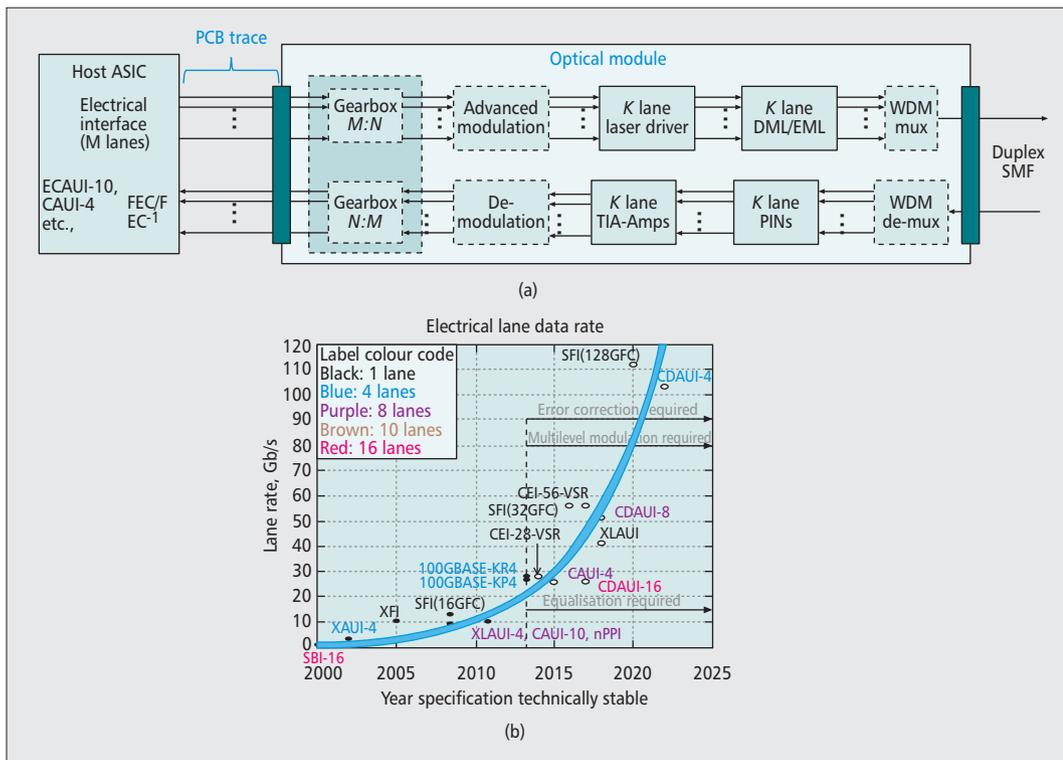
**Figure 1.** a) Diagram of a high-speed Ethernet including electrical interface and optical module; b) trends for standards-based electrical interfaces. Filled circles indicate developed, while empty circles represent under development or discussion.
