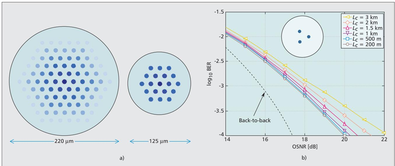
**Figure 5.** a) High-density hexagonal-core MCFs with 91 and 19 cores in a 220 and 125  $\mu\text{m}$  diameter fiber, respectively. b) Bit error-rate (BER) as a function of optical signal-to-noise ratio (OSNR) after 1000-km transmission over a 3-core MCF having different coupling lengths  $L_c$ . A single channel is launched in each of the three cores with 7 dBm average power (from [13]).
