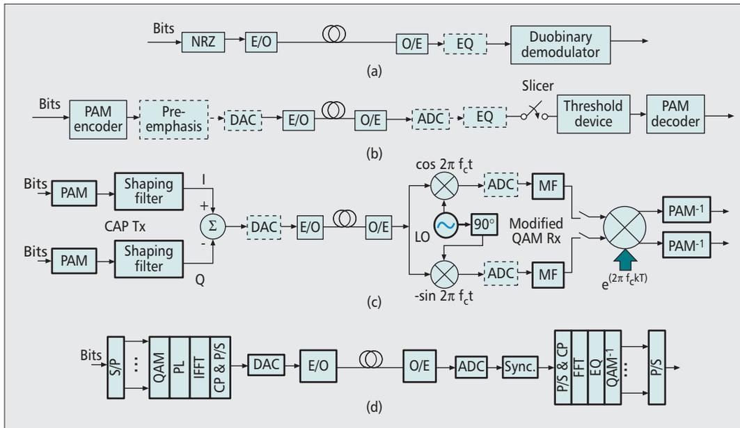
**Figure 3.** System diagram of an optical data link using: a) duobinary; b) PAM; c) hybrid CAP/QAM; d) QAM-OFDM. E/O: electrical-to-optical conversion; EQ: equalizer; MF: matched filter; PL: power loading; P/S: parallel-to-serial conversion; CP: cyclic prefix; Sync: synchronization; (I)FFT: (inverse) fast Fourier transform; DAC/ADC: digital-to-analog/analog-to-digital conversion.
