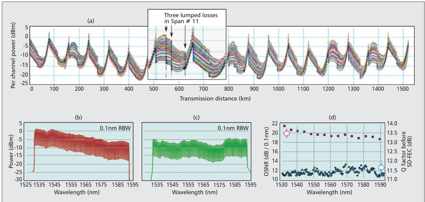
**Figure 6.** a) Results of the  $150 \times 100\text{G}$  all-Raman field trial, simulated per channel power profiles; b) spectrum at the booster output; c) spectrum after 1504 km transmission; d) measurements of OSNR and Q factor across the  $150 \times 100\text{G}$  channels spaced at 50 GHz.
