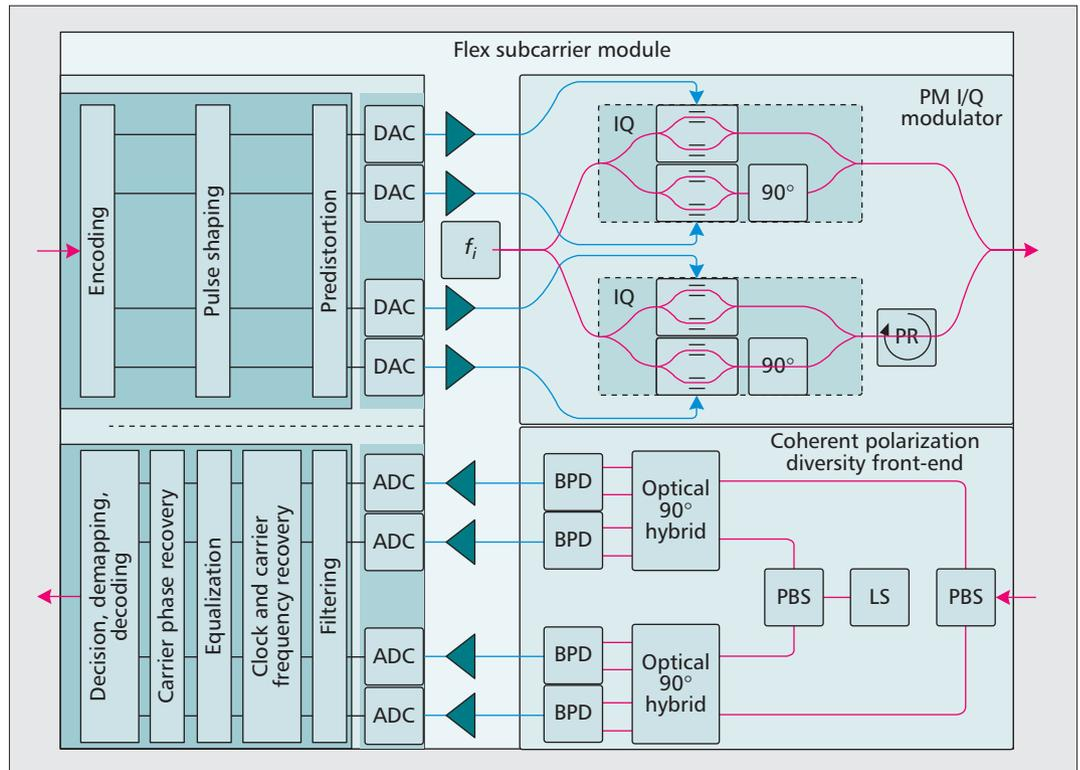
**Figure 3.** Flex subcarrier module building blocks.
