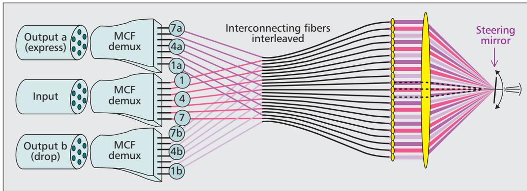
**Figure 2.** A single mirror can simultaneously steer multiple beams that impinge on it at different angles of incidence. In a WSS, there are many such mirrors, one for each wavelength. In this illustration, spatial modes from multi-core fibers are converted to single-mode fiber signals in the component labeled MCF demux (after [3]).
