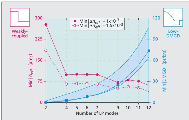
**Figure 2.** Min  $|A_{eff}|$  at 1550 nm of step-index weakly coupled FMFs for  $\text{Min}|\Delta n_{eff}| = 1.0$  and  $1.5 \times 10^{-3}$  (red circles) and  $\text{Max}|\text{DMGD}|$  at 1550 nm of trench-assisted graded-index low-DMGD FMFs (blue squares for optimized designs, blue area delimiting the lowest and highest values of concatenations taking process variability into account) as a function of the number of LP modes. Lines are guides for the eye.
