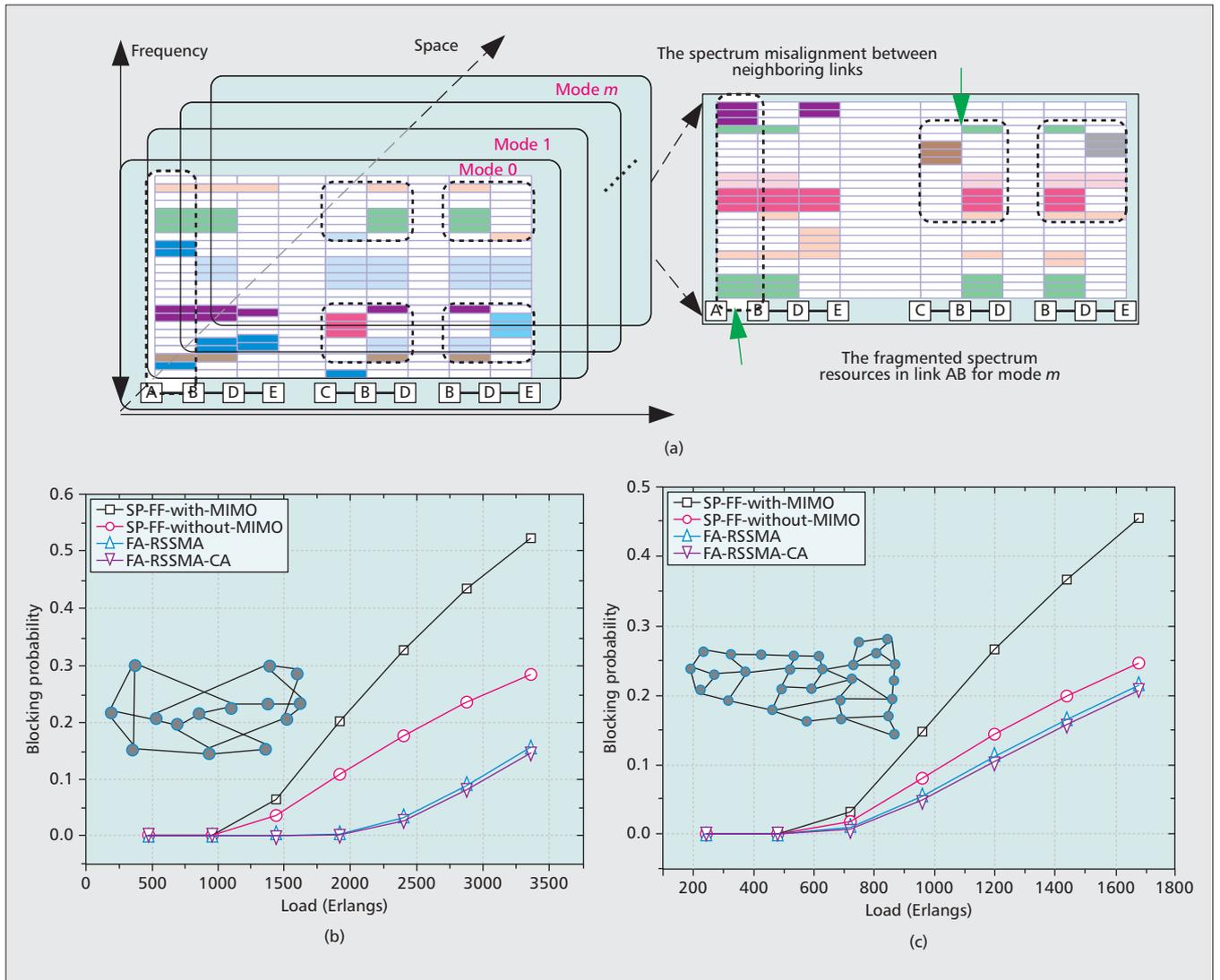
**Figure 5.** a) Spectral fragmentation on the spectral-spatial-temporal dimensions; b) blocking probability comparison of different algorithms in the 14-node NSFNET network; c) blocking probability comparison of different algorithms in the 28-node USBN network.
