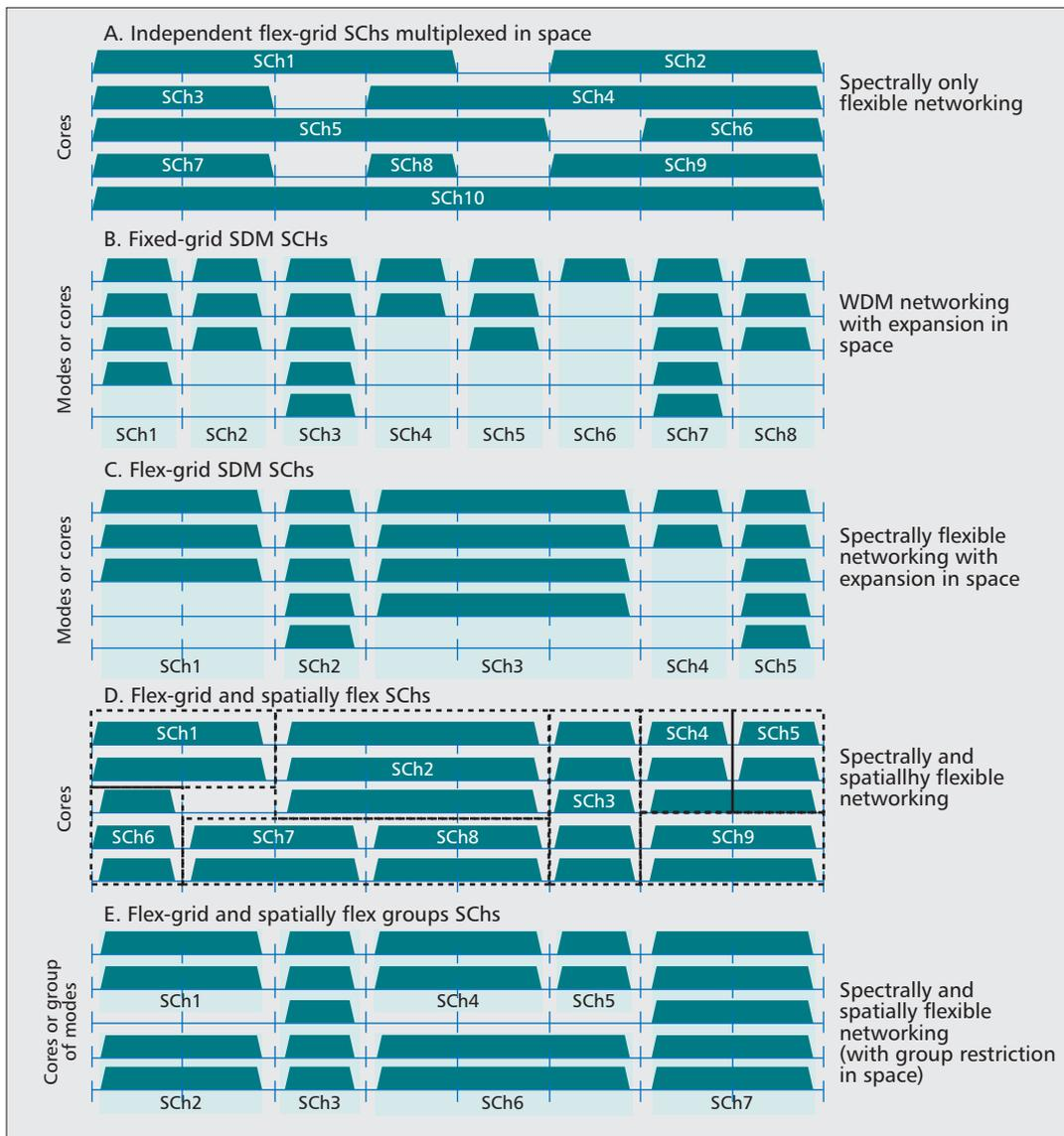
The channel allocation flexibility increases significantly with the introduction of the space dimension. However, the key question from the networking point of view is: What added value could the space dimension bring to the flexible optical networking concept?
