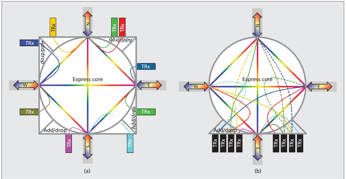
**Figure 2.** Schematic ROADMs designs: a) basic design; b) colorless/directionless/contentionless and flexible grid (CDC-F) design for flexible optical networks (dashed lines represent potential connections).
