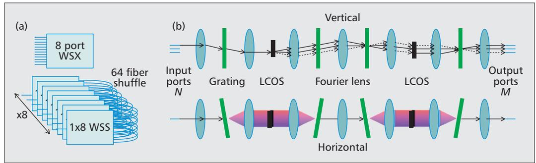
**Figure 3.** a) Functionality of a wavelength selective cross connect built using many WSSs and fiber shuffle; b) schematic of the optical arrangement for an  $N \times M$  wavelength crossconnect [2].
