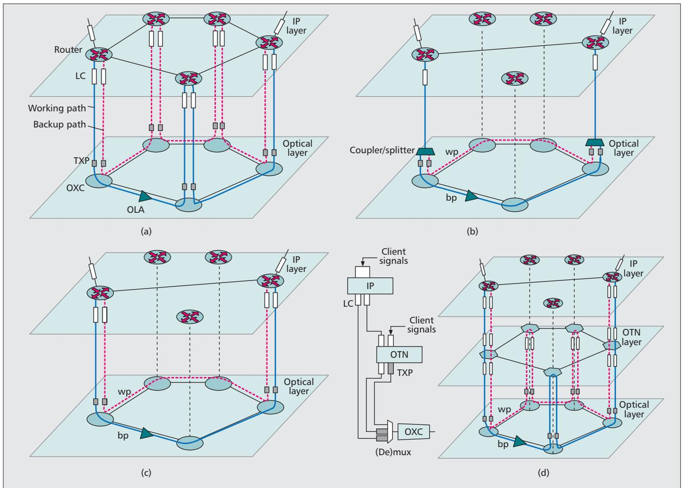
**Figure 1.** a) 1+1 protection at the IP layer; b) 1+1 protection at the optical layer; c) employing optical bypass at the IP layer; d) grooming at the OTN layer. LC: line card, TXP: transponder, OXC: optical cross connect, OLA: optical line amplifier, wp: working path, bp: backup path.
