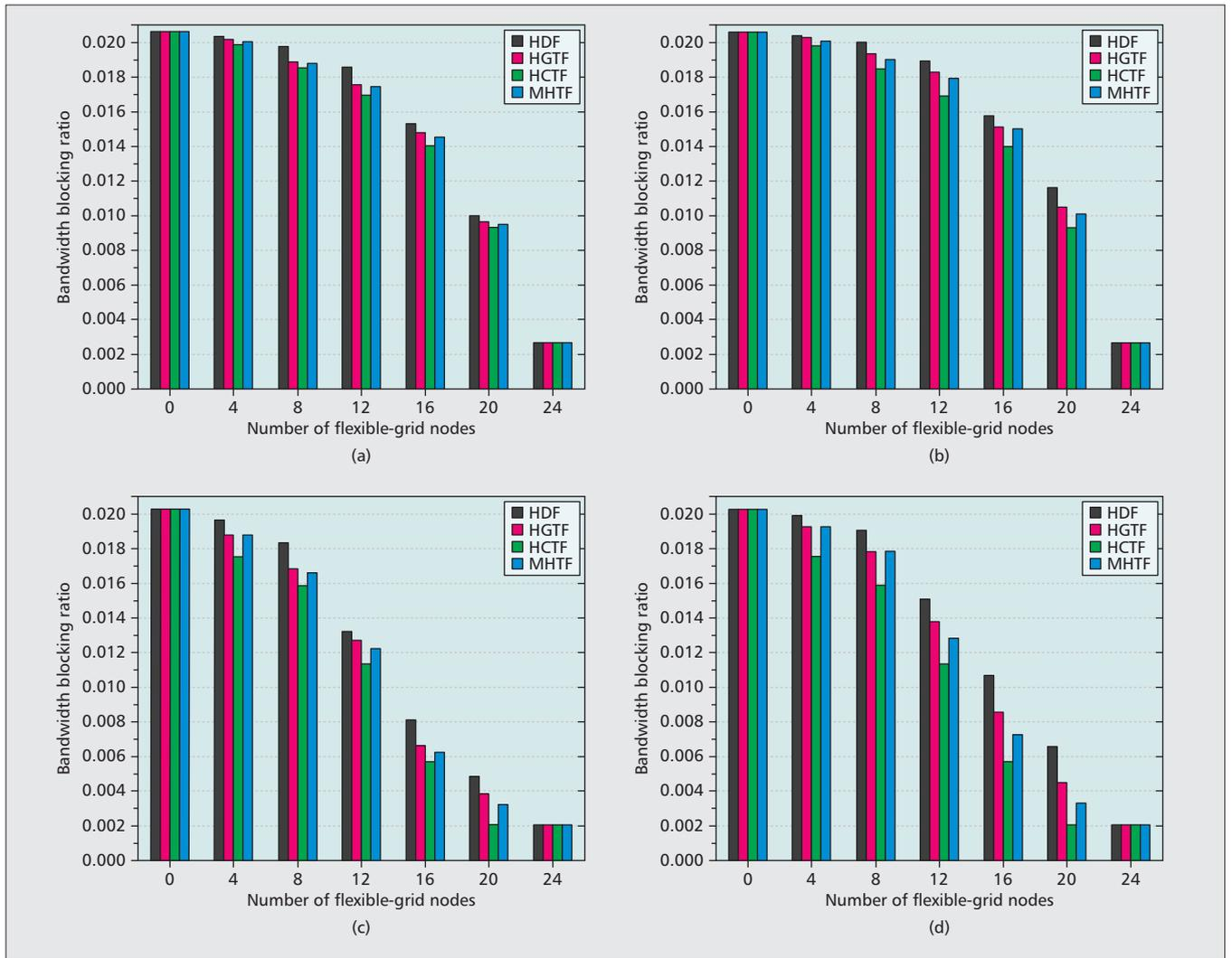
**Figure 5.** Bandwidth blocking ratio for traffic profile 3: a) forming one island under uniform traffic; b) forming two islands under uniform traffic; c) forming one island under non-uniform traffic; and d) forming two islands under non-uniform traffic.
