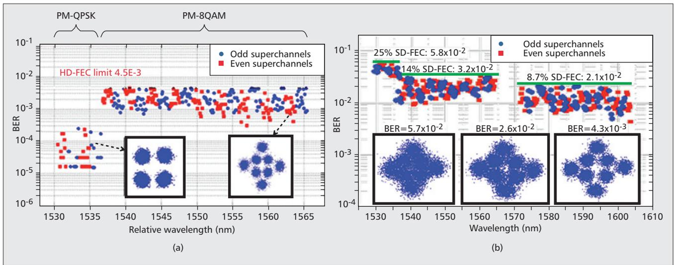
**Figure 5.** a) Field trial results of high capacity flexible transponders with adjustable modulation formats and b) adaptive FEC overheads.
