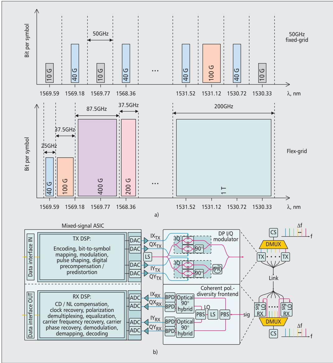
**Figure 1.** a) Fixed (50-GHz granularity) vs. Flex-grid optical systems (12.5-GHz granularity); b) block diagram of a Flex subcarrier module. ASIC: application-specific integrated circuit (ASIC); TX: transmitter; DP: dual-polarization; DMUX: demultiplexer; RX: receiver; LS: light amplification by stimulated emission of radiation (LASER) source; LO: local oscillator; BPD: balanced photo-detectors; CS: comb source; NL: nonlinearity.
