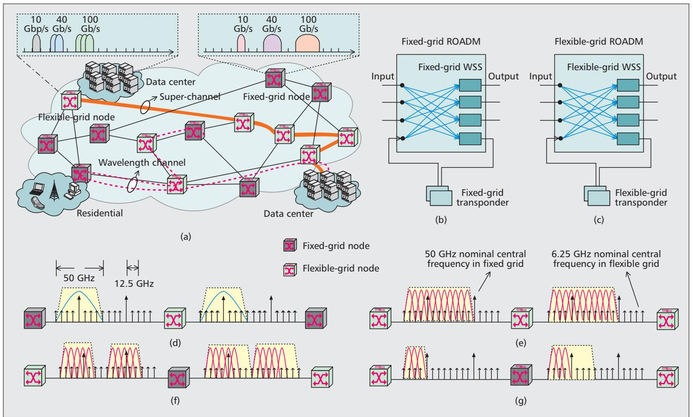
**Figure 1.** Optical network with co-existing fixed-grid and flexible-grid technologies: a) network architecture; b) fixed-grid ROADM; c) flexible-grid ROADM; d) wavelength channel; e) 200-Gb/s super-channel; f) two 100-Gb/s channels; g) 40-Gb/s subchannel.
