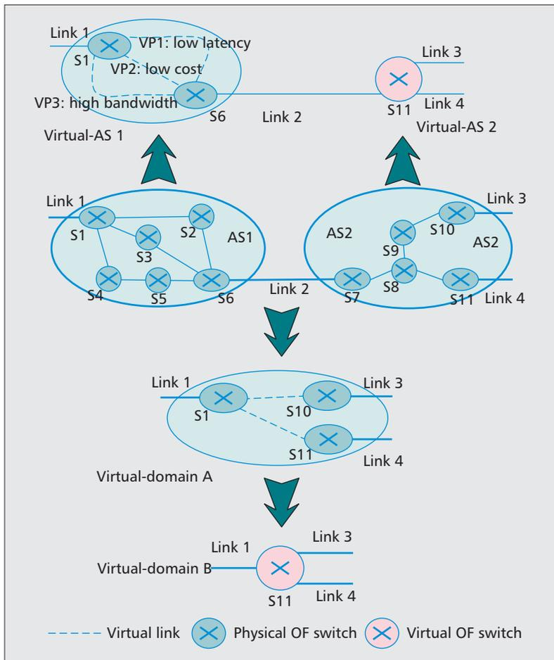
**Figure 2.** Network view virtualization (VP: virtual path; OF: OpenFlow; S: switch).
