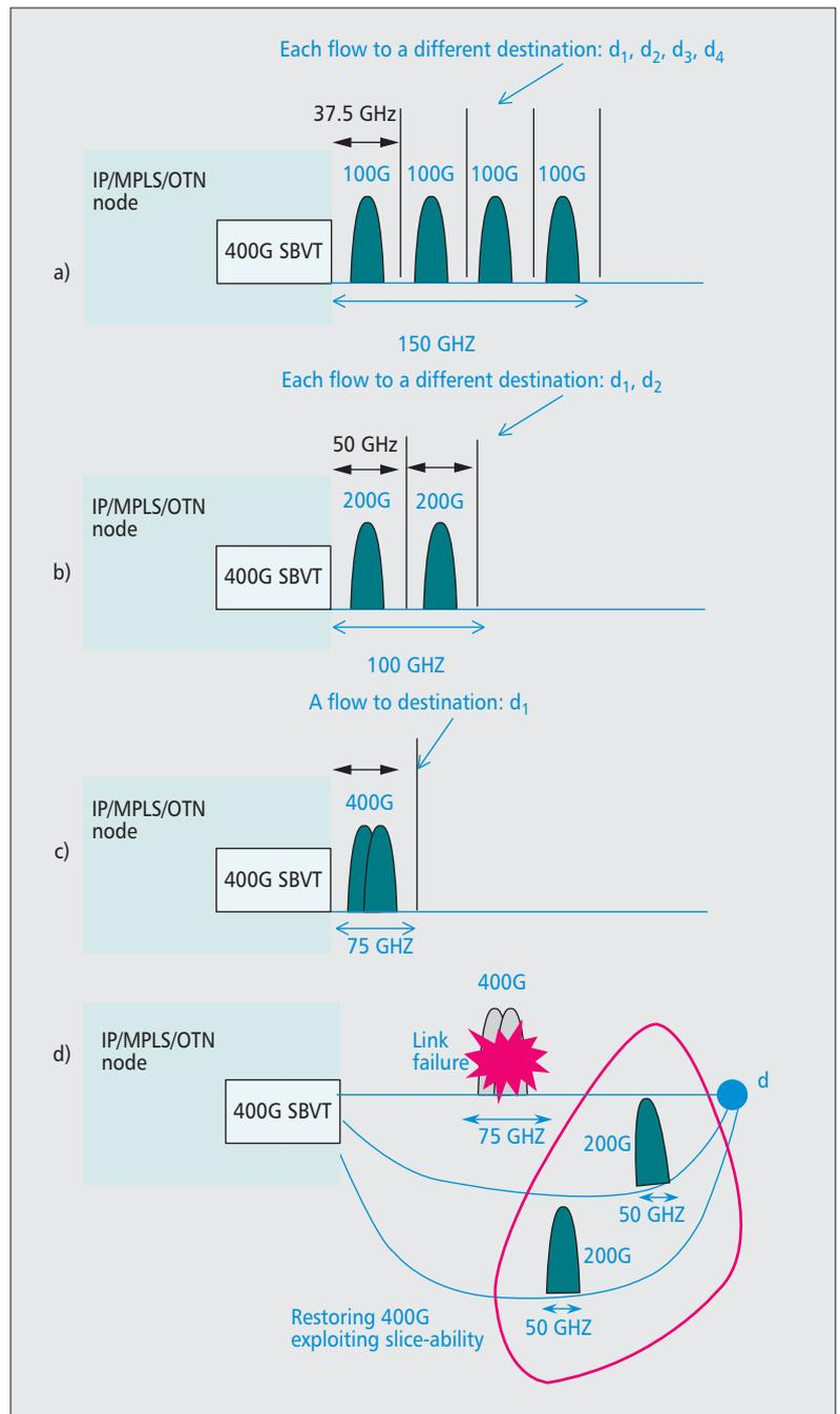
**Figure 5.** a)–c) Flexible utilization of an S-BVT by varying the bit rate per destination; d) sliceability used in restoration.
