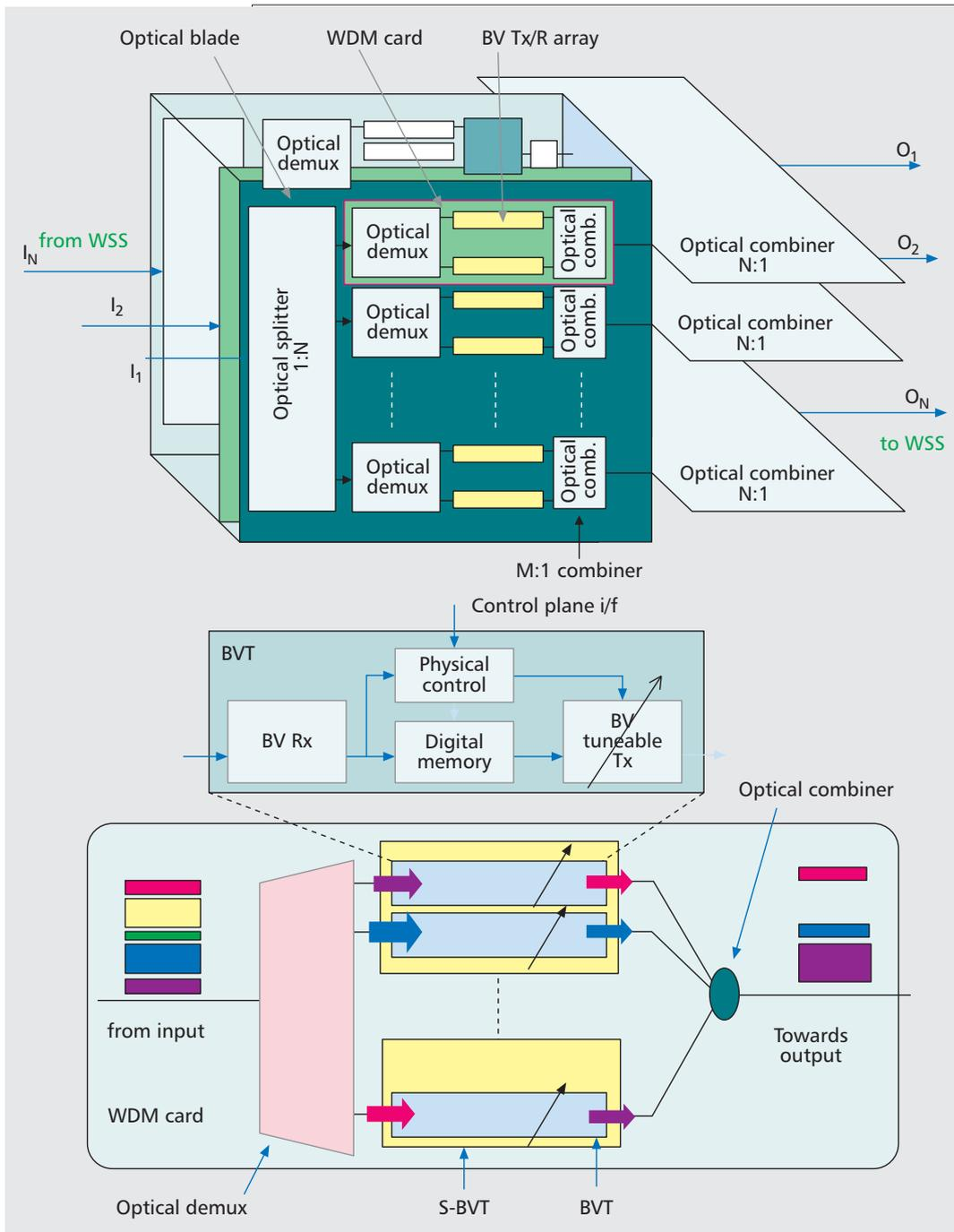
**Figure 4.** a) Overview of the SERANO architecture; b) details of the WDM card and the S-BVTs.
