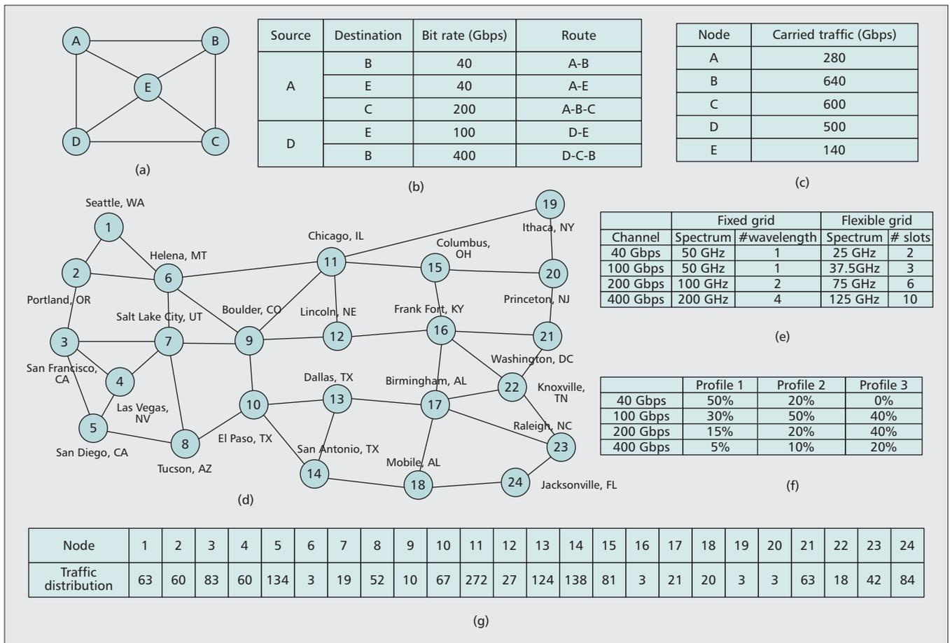
**Figure 2.** a) 5-node topology; b) traffic matrix; c) carried traffic by each node; d) U.S. network topology; e) optical channels in fixed-grid and flexible-grid technologies; f) connection demand ratios in different traffic profiles; g) traffic distribution in the non-uniform case.
