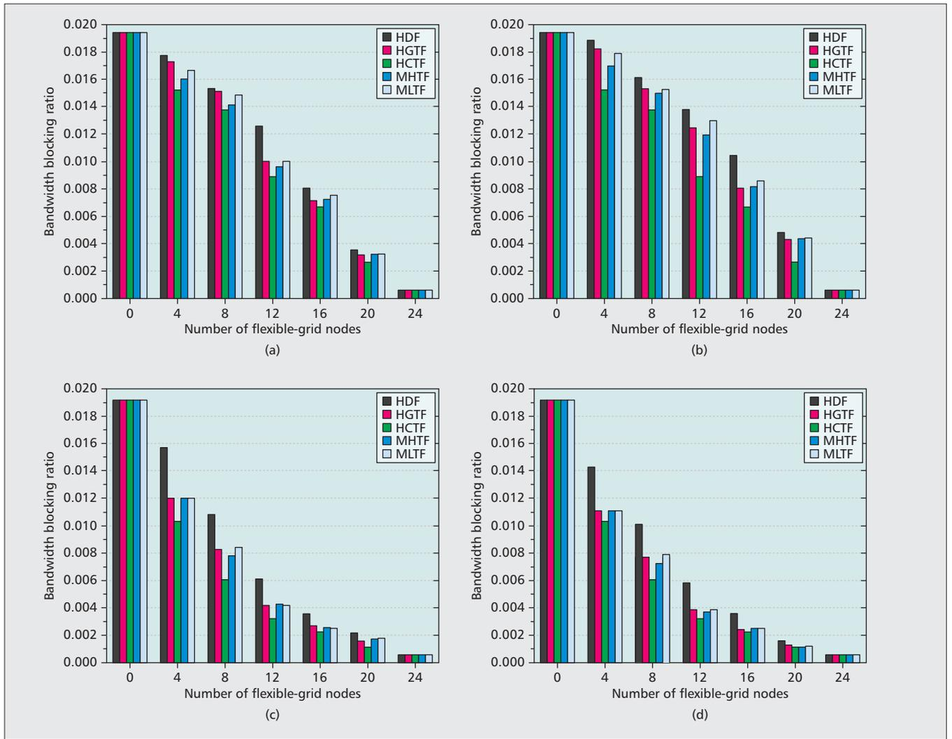
**Figure 4.** Bandwidth blocking ratio for traffic profile 2: a) forming one island under uniform traffic; b) forming two islands under uniform traffic; c) forming one island under non-uniform traffic; and d) forming two islands under non-uniform traffic.
