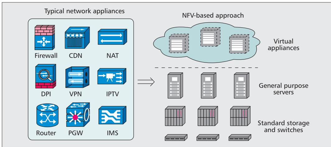
**Figure 1.** From dedicated hardware-based appliances for network services, such as firewalls, content delivery networks (CDNs), network address translation (NAT), deep packet inspection (DPI), virtual private networks (VPNs), IPTV, routers, packet data network gateways (PDN-GWs or PGWs), and IP multimedia subsystems (IMSs), to software-based NFV solutions.
